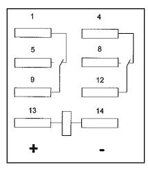
5.10 - Model 21H High-Density Flash Transfer Relay (HDFTR) Pin-outs
